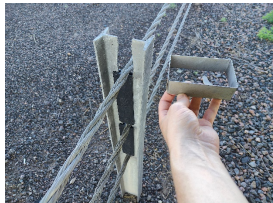
Figure 2-12 – Broken steel rings (typ.)
